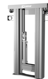
Triplex full free lift, free visibility
