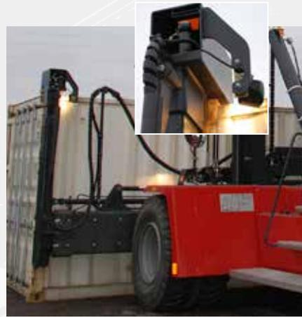
The levelling function on the twistlock attachment is enabled by the mobility of each twistlock. This gives a simpler construction which offers increased reliability and easier servicing.
