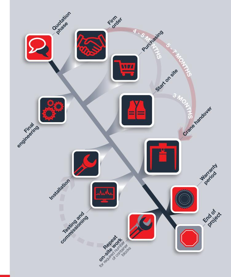
This is an overview of a typical electrification project, the phasing and an estimate of the time for each phase. These timings are approximate and actual timings will depend on the scope of the project, the number of RTGs and the specific requirements of each terminal.
